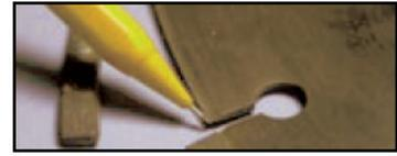
**Cause:** Undercutting is a condition in which the steel center wears faster than the diamond segment, especially in the areas where the segment and core are joined.
