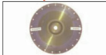
**Cause:** The bond is too hard for the material being cut. The hard bond retains the diamonds, and they begin to round off, causing the blade to become dull. Instead of cutting, the blade begins to “pound”, causing the blade to wear out-of-round.
